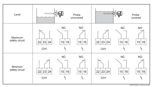
Function of the limit indicator dependent on the level and fail-safe circuit.
